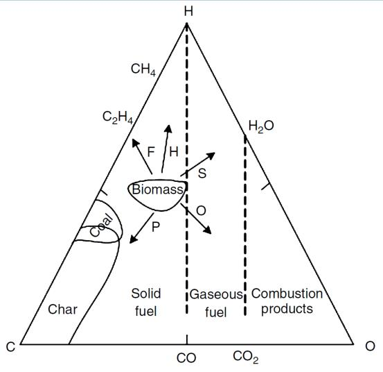
H hydrogen S steam O oxygen P slow pyrolysis F fast pyrolysis L lignin C cellulose/hemicellulose
