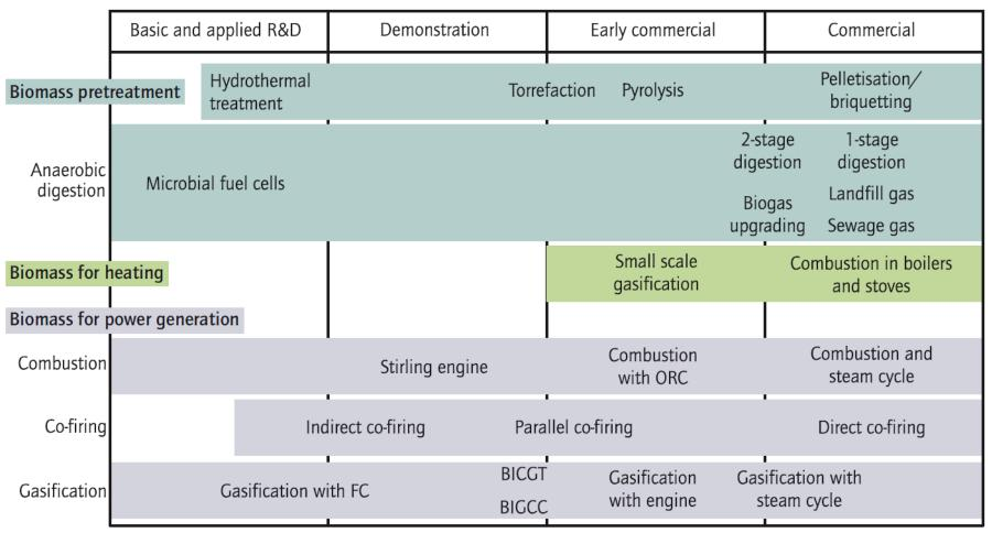
Note: ORC = Organic Rankine Cycle; FC = fuel cell; BICGT = biomass internal combustion gas turbine; BIGCC = biomass internal gasification combined cycle
