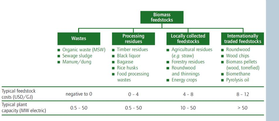
Examples of different biomass feedstocks, typical feedstock costs, and plant capacities
